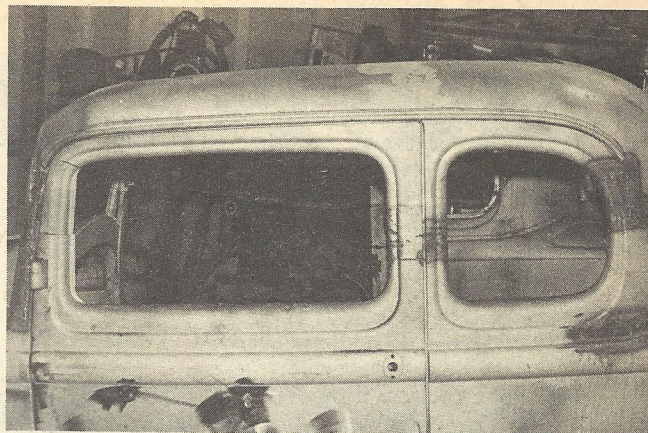
A cut is made along upper front corner and the door posts are aligned before welding.
