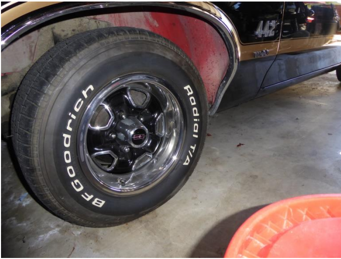
Radial T/A's all around on correct Olds rally wheels. All trim rings, caps and wheel hardware are very good. Notice the read fiberglass inner fender aprons. These are a W-30 feature. This car has enough of the W-30 items that it does a great job of representing the W-30 optioned 442.
