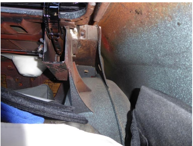
Leather These photos are shared so some view of the inner "back-side" of rear panels can be seen. These areas show the bottom area of the rear window that on some cars will show rust repairs. This car appears to have no issues or repair and is in very goods condition.
