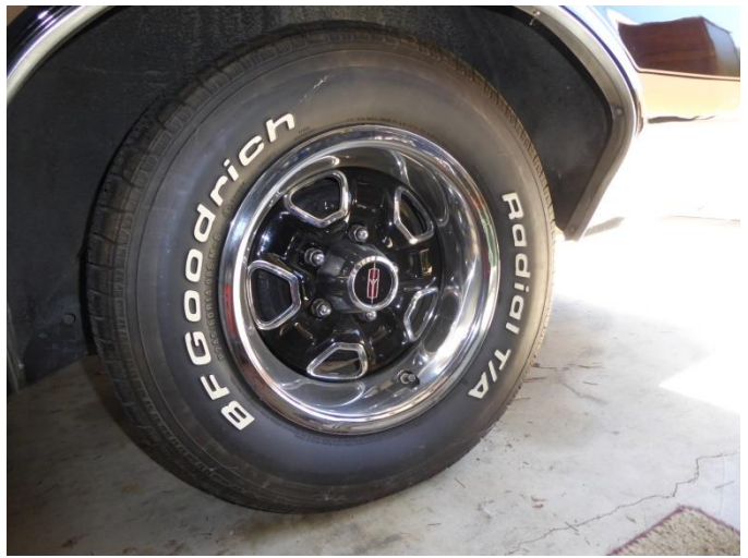
Radial T/A's all around on correct Olds rally wheels. All trim rings, caps and wheel hardware are very good. Notice the read fiberglass inner fender aprons. These are a W-30 feature. This car has enough of the W-30 items that it does a great job of representing the W-30 optioned 442.
